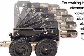
For working in larger pipes, adjustable elevators and larger wheels provide coverage of a range of pipe sizes, while the powered elevator enables fine, remote adjustment, ensuring compliant centering in pipes from 12"/305mm to 36"/900mm).
