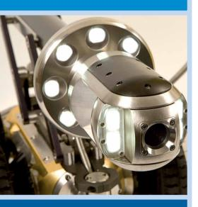
Auxiliary lighthead provides additional lighting for large or dark pipes.
