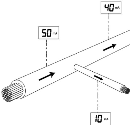
Figure 7.3 Current readings
