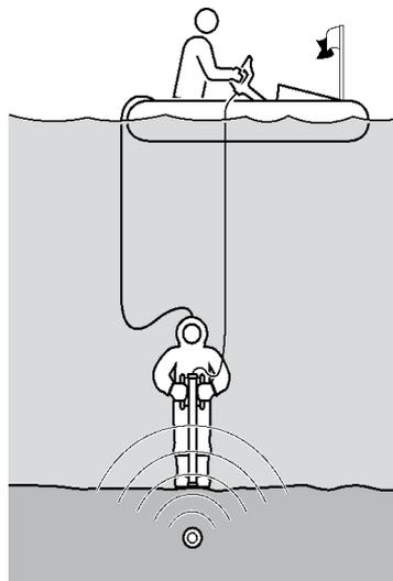
Figure 12.10: Using a submersible antenna
