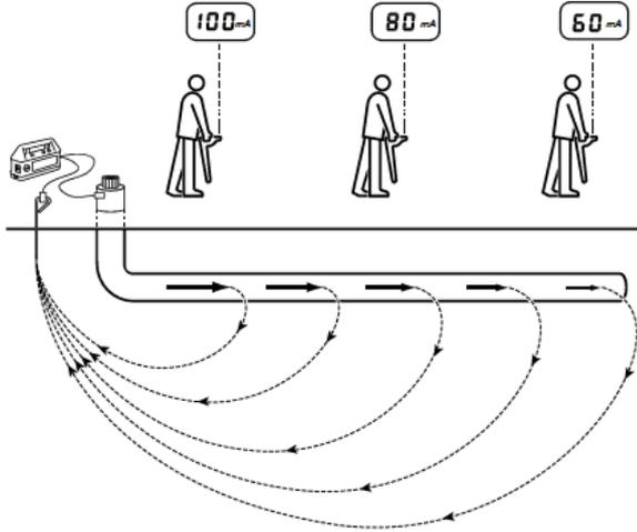
Figure 7.7: Current readings using transmitter signals
