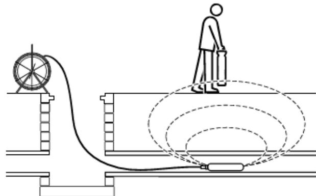
Figure 12.6 Sonde deployment
