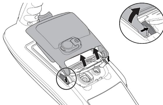
Figure 4.4 Press the retaining latch inwards
