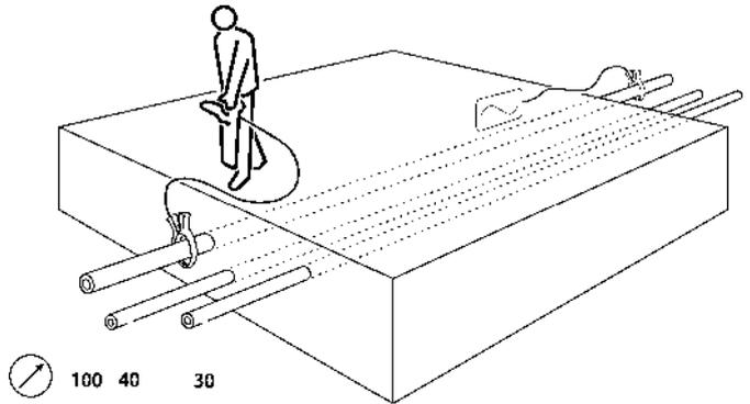
Figure 12.1: Connecting clamps
